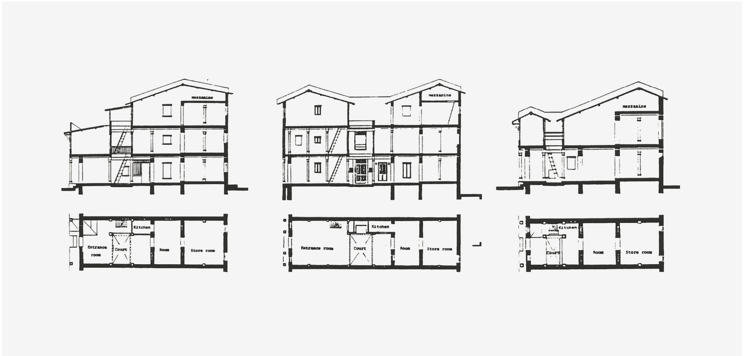
Cross sections of three traditional houses in Ahmedabad, India- From Nagarkatti, Arjun. "An Intervention in an Extant Situation : A Guideline Case-Study - Ahmedabad, India." (Thesis, Massachusetts Institute of Technology, 1984), 17.
