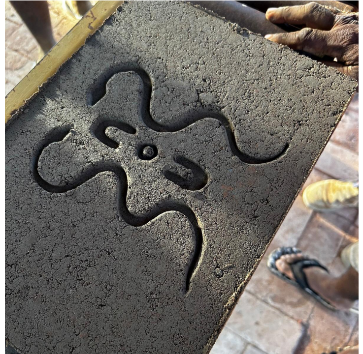
The Wilya Janta team collecting termite mounds to make mud bricks. Each brick is stamped with the Wilya Janta logo—two snakes—symbolizing their approach to working across Indigenous and non-Indigenous knowledge systems. Photographs by Andrew Quilty, 2023.
