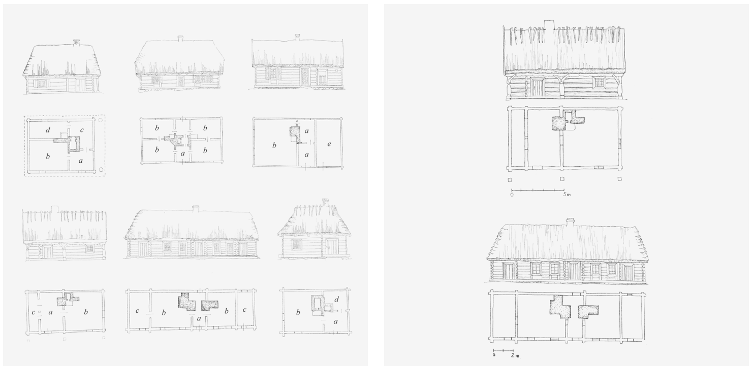
Different types of peasant homesteads. a. vestibule b. chamber c. compartment d. bed chamber e. stable. Drawn by the author, adapted from Czerwiński, Budownictwo ludowe w Polsce , 50–59.
