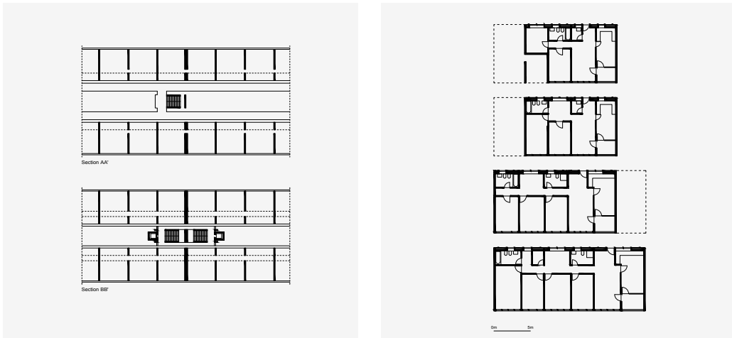
Mario Fiorentino and collaborators, Housing at Corviale, Rome, 1972-1981, diagram showing circulation and load-bearing structure. Vertical core apartments (below), gallery apartments (top). Drawing by Romain Barth.
