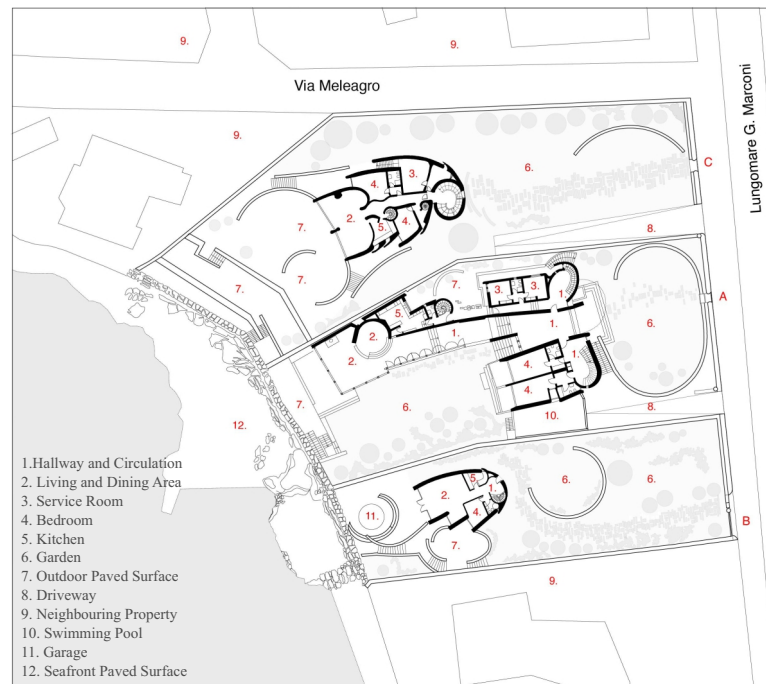
Siteplan of 'Villa Triptych' illustrating the ground floor. Redrawing by the author. Original drawings from Archivio Centrale dello Stato (ACSRo) Fondo Luigi Moretti, Rome. A. Villa La Saracena (1953-57), B. Villa La Califfa (1961-67), C. Villa La Moresca (1970-81).
